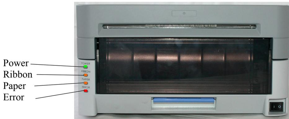
The flashing LED indicates the printer status
