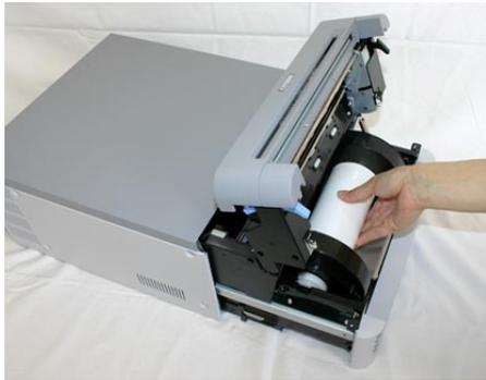
3. Cut off any partially printed, wrinkled, or otherwise inferior paper evenly with a pair of scissors, and reset the paper. If wrinkles or partially printed areas are left, it could cause the paper to jam again.
