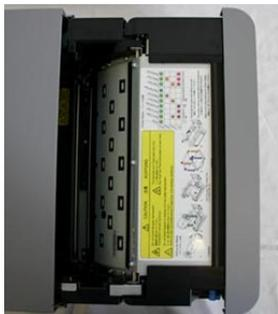
1. Pull any paper remaining in the printer in the direction shown, and cut off any wrinkled or partially printed areas evenly with scissors.
