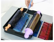
Carefully remove any ribbon remaining in the mechanism. Any pieces of ribbon left inside the mechanism could affect print quality. In this case, clean the platen roller see P.27
