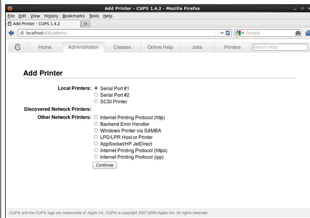
If the serial port to connect the printer is shown in the port list, choose the port (Ex. Serial Port #1) and press "Continue".
