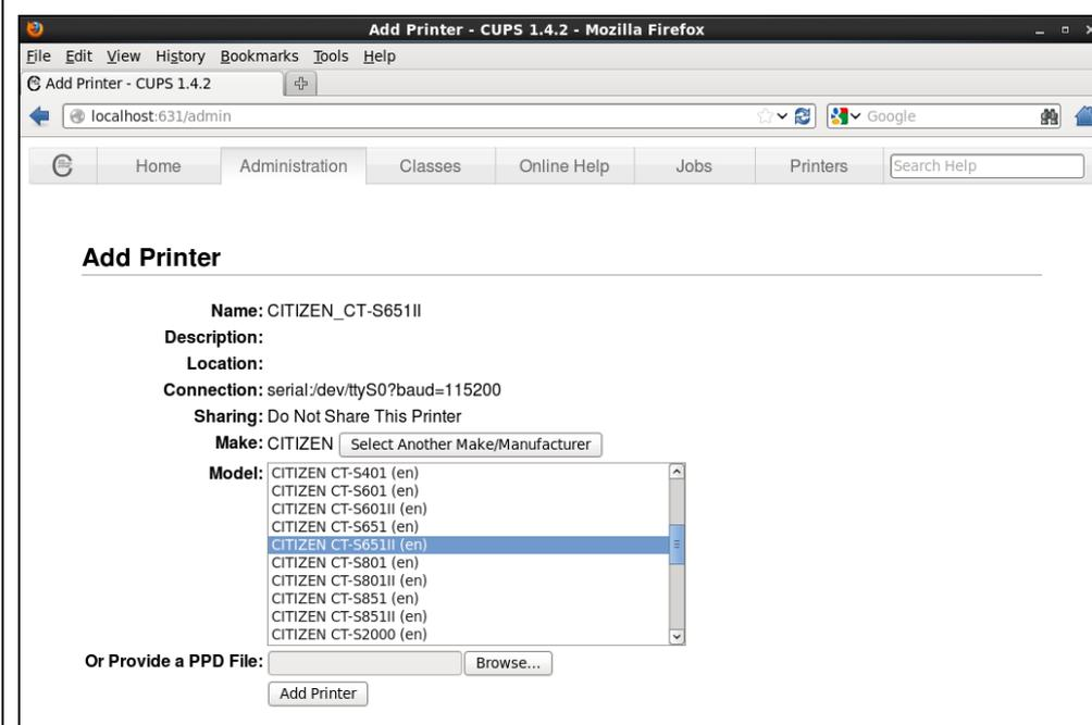
Choose the model to install in the "Model" list and press "Add Printer" button. This will end the printer driver installation and move to "Set Default Options" menu.
