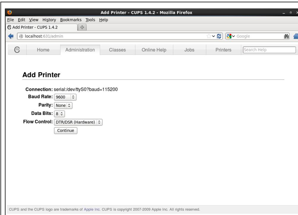
When serial port setting menu is shown, choose the setting to match the serial port of the connected printer. (Serial port setting of the printer can be checked by self printing.) Press "Continue" button.
