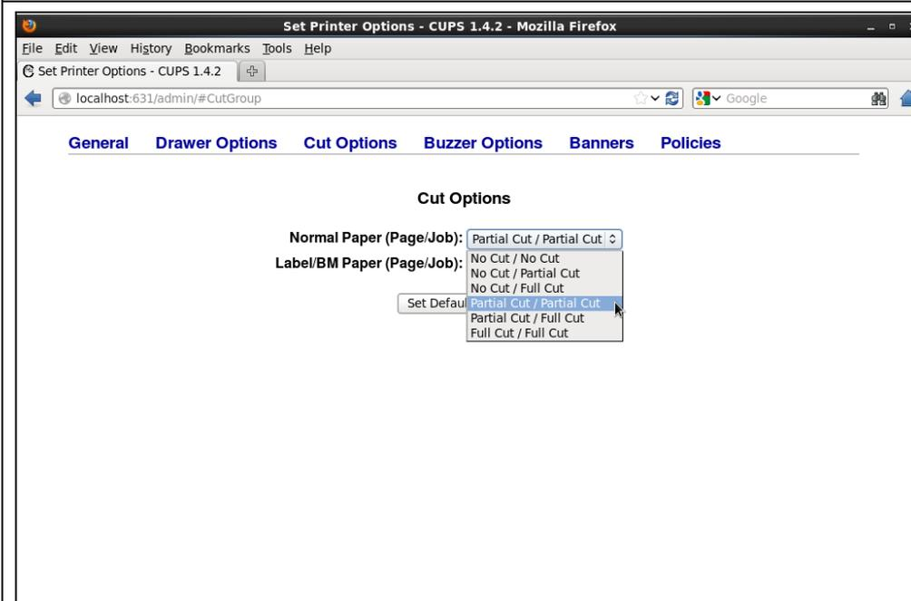
For the normal paper, there can be maximum 6 different cutting method combinations by partial cut, full cut and no cut.
