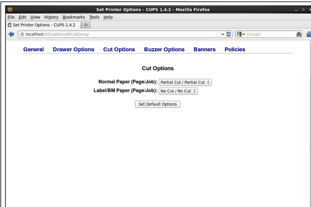
Cutting method for middle page end (Page) and cutting method for receipt end (Job) can be chosen.
