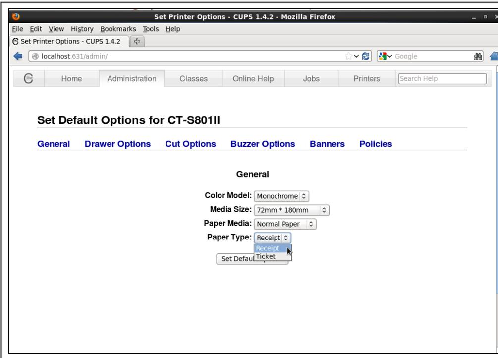
You can choose Receipt or Ticket as paper types. Receipt allows flexible paper length according to the data length to avoid waste of paper. Ticket print in fixed length even the print data is short.
