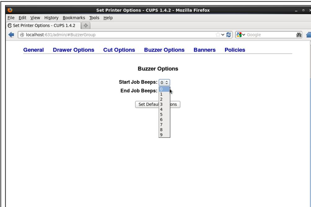
The timing of buzz can be selected from top of receipt (Job Start) or end of receipt (Job End). Number of buzz can be selected from 1 to 9. Default setting is no buzz.
