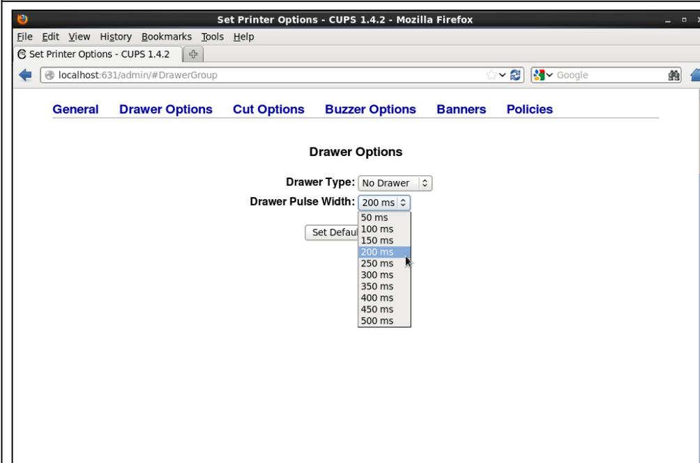
Usually, it is not necessary to adjust the pulse to send to cash drawer but when necessary, change the value.
