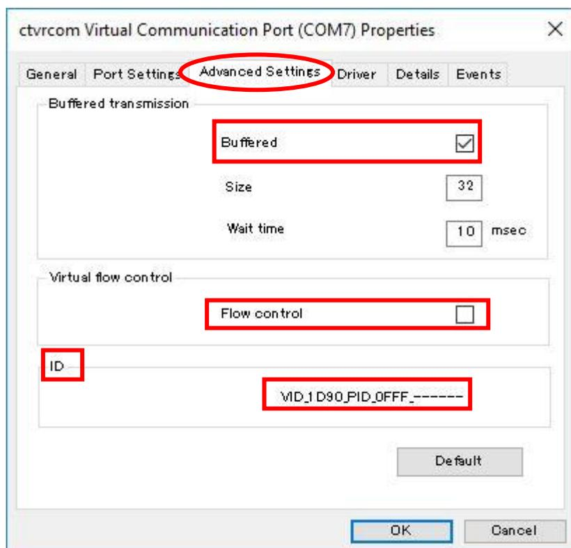
**ID:** Although USB identifies the communication partner by ID, since different virtual COM IDs (two types) are assigned to the printer depending on the model; COM7 and COM8 are prepared as port numbers to which each USB ID is assigned.
