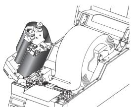
Ribbon Tension Adjustment (p.61) Ribbon Balance Adjustment (p.63) 6. Push the head close knob to lower and lock the head unit. Be sure to always push the head close knob to lock the head unit. If the ribbon is wrinkled, push the Feed key until the wrinkles disappear. If the wrinkles do not disappear or if it slips, perform ribbon balance adjustment and ribbon tension adjustment. See "Chapter 3 Printer Adjustments" for these adjustment methods.
