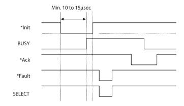
**Note:** If the \*Init signal does not have width of 10 to 15µsec or more, it cannot act as an Init signal. If it is lower, the \*Init signal is ignored. BUSY starts up when the \*Init signal is perceived.
