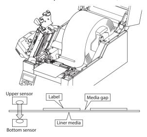
3. If the Pause key is pressed then released while the Feed key is continually pressed, the sensor is automatically adjusted.
