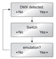
By selecting "Yes" the printer will reboot and automatically switch to Datamax® emulation (DM4/DMI/DPP). The printer will return to the Ready status if "No" is selected.
