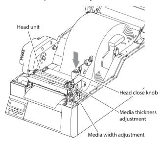
9. With the power switched on, push the Feed key to feed the media.
