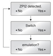
By selecting "Yes" the printer will reboot and automatically switch to ZPI2 emulation. The printer will return to the Ready status if "No" is selected.
