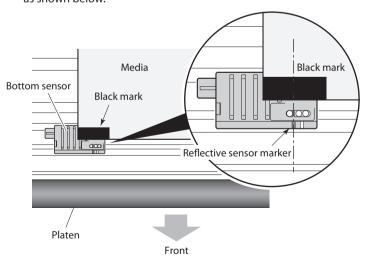
\* When using a reflective sensor, install the upper sensor in such a manner that the upper sensor marker is not in the same position of the reflective sensor marker. Paper end detection may be impossible if installation is not done in this manner.
