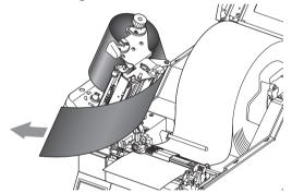
4. Using the adhesive leader of the ribbon or some adhesive tape, fix the ribbon that you have pulled out on the ribbon holder on which the paper core has been set and wind it on the ribbon holder.
