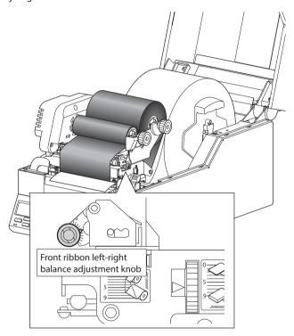
1. Look at the ribbon from font side and check on which side (adjustment knob side /the side opposite to the adjustment knob) loose is present between the ribbon on the feeding side and ribbon guide shaft on the back side.
