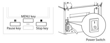
2. After "Sensor Cal Mode" lights up, release the keys to change the printer to sensor adjustment setting mode.
