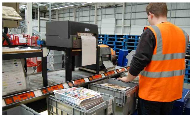
The CLP 8301 features **all-metal construction** making it a durable solution for industrial environments, in addition to a **Hi-Lift™ mechanism** that minimises the space needed to install it, and makes it simple to load media or ribbons, leading to less downtime and errors. The printer's internal **200mm media capacity** enables full size rolls to be kept within the heavy-duty metal case, protecting the media from dust and dirt and resulting in consistently high quality printing.
